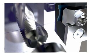
Alignment stop made of cheap rectangular symmetrical plates with a quick change system.
